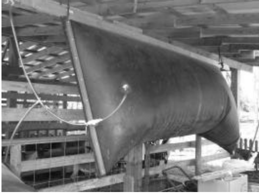
Figure 4. Flotation type storage tank. (Also see ECHO's Concept Papers "Technologies Demonstrated at ECHO: Floating Drum Biogas Digester.")
