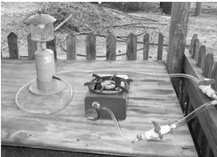
Figure 5. Gas from the storage container can be used in salvaged gas stove burners or any similar locally fabricated device. Gas may also be used in any common pressure lamp after its fuel orifice has been modified.
