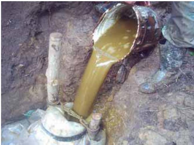
*Left: Initially charge your bio-digester with up to 20 buckets of manure mixed with water. After this the digester requires only 2 buckets of charge each day.*
